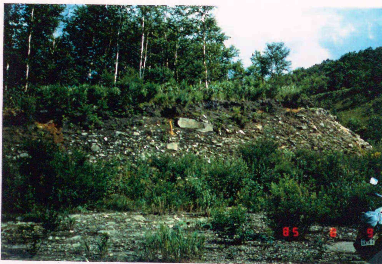
Photo 1 Section at Loc. 42. Slope deposits, more than 1-5 m thick, are underlain by Ta-d. Measure is 1 m long.
