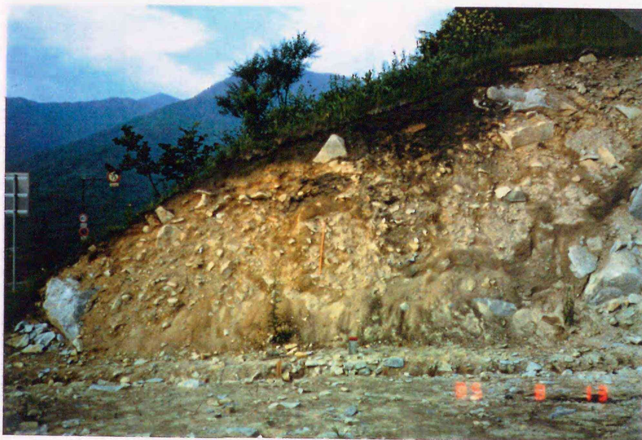
Photo 7 Section at Loc. 45. Slope deposits are intercalated with Ta-d at depth of 70-80 cm. Measure is 1 m long.
