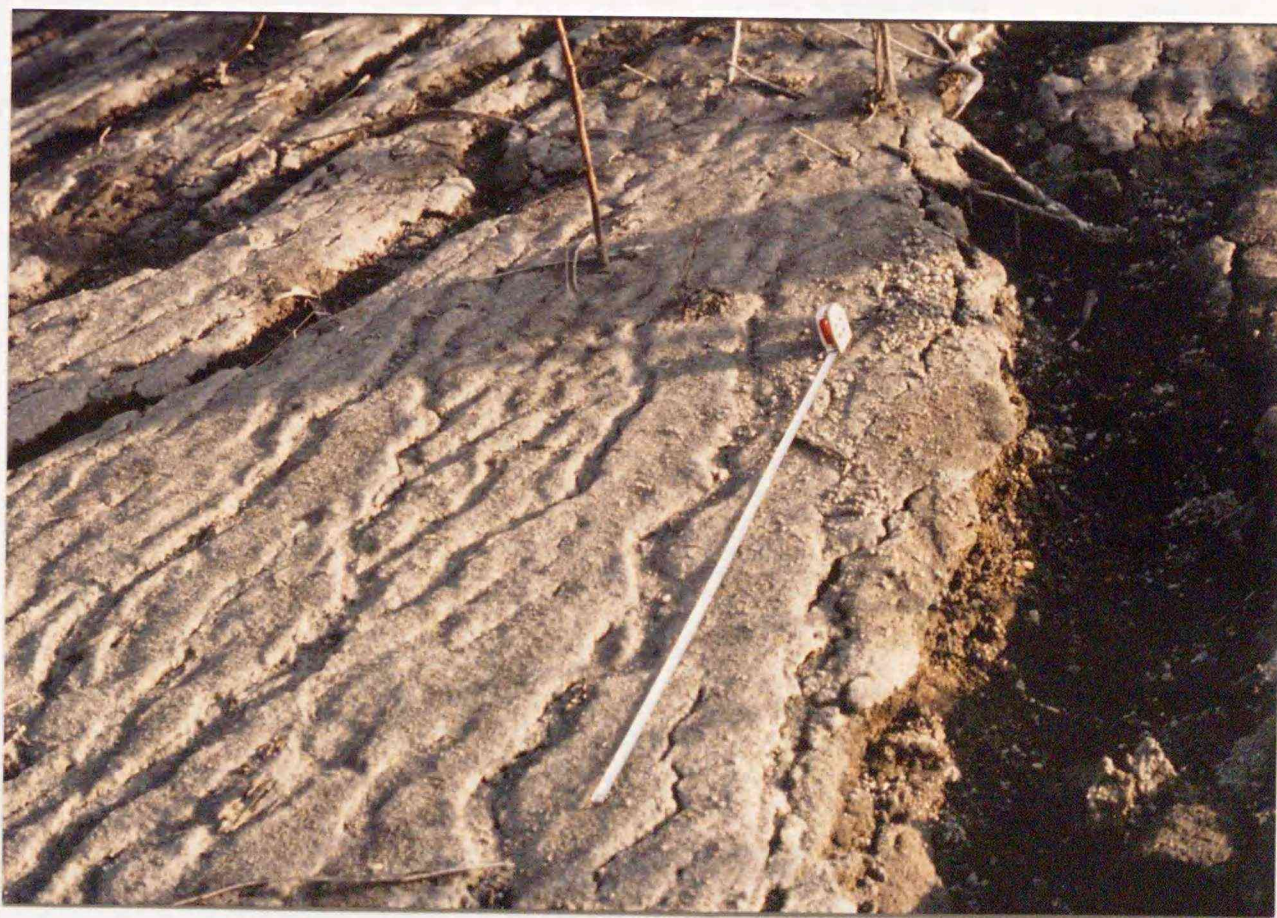
Photo 2-2 Rills and gullies formed on the experiment slope.
