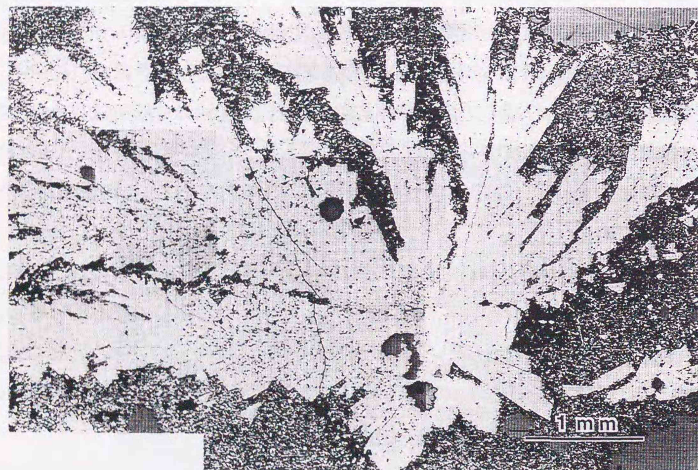
Fig. 3.5 Morphology of 123 phase which was cooled from 1000°C to 950°C of a cooling rate of 30°C/h.
