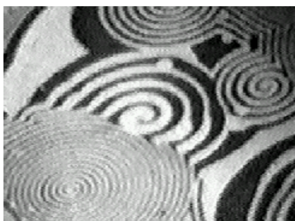
Fig. 1. PEEM image of CO oxidation on a Pt(110) surface at 450 K with P_{O_2}=4 \times 10^{-4} mbar and P_{CO}=4 \times 10^{-5} mbar. Dark and grey regions are oxygen and CO adsorbed regions, respectively. 3
