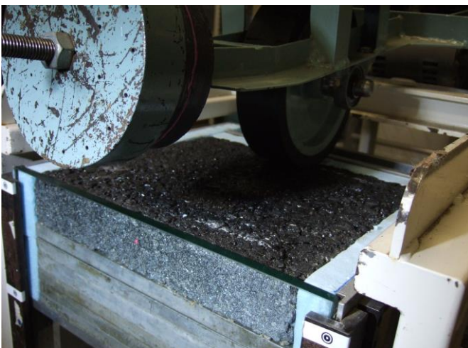
Photo 1. Overview of wheel tracking test of Hokkaido University Type
