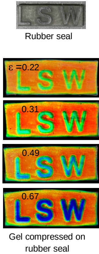
Figure 8: Rubber seal engraved with LSW (top most) and the change of color display of PDGI/PAAm gel sheet, being compressed on the seal, through engraved ‘LSW’ from yellowish green to blue upon increasing strain (top to bottom). [Reproduced with permission from Ref. 19].
