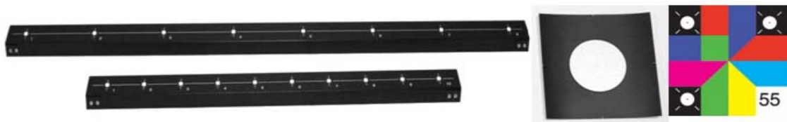
図 2.3 Scale Bar (left), Reflective target (middle), Color-Coded target (right).
