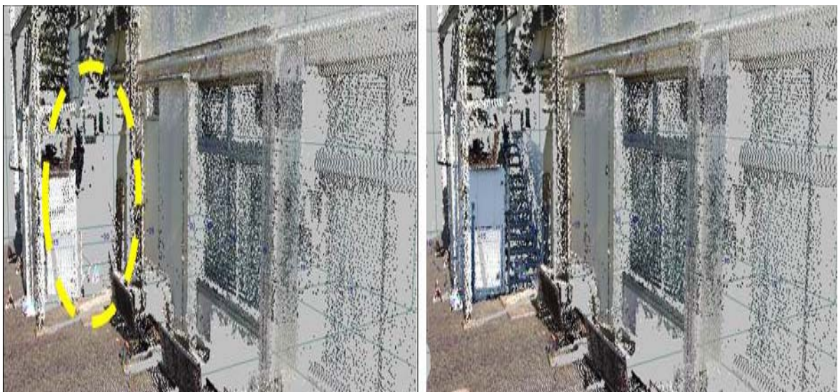
図 3.18 Model integration : Before integration (left), After integration (right)
