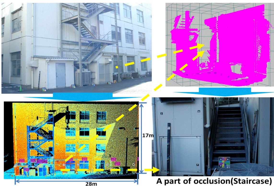
図 3.2 A building to be measured: Photograph (top left), Point- cloud (top right, bottom left), Measuring image (bottom right).
