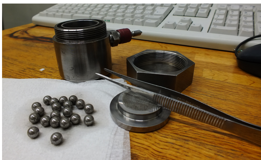
Figure 2.1: A picture of the set of ball-milling pot and balls.
