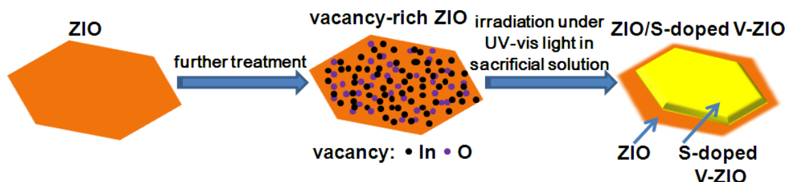
Figure 2.1 Schematic of the formation process of ZIO/S-doped V-ZIO composite.
