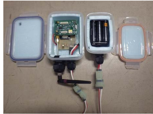
Figure 2: Constant power supply system
