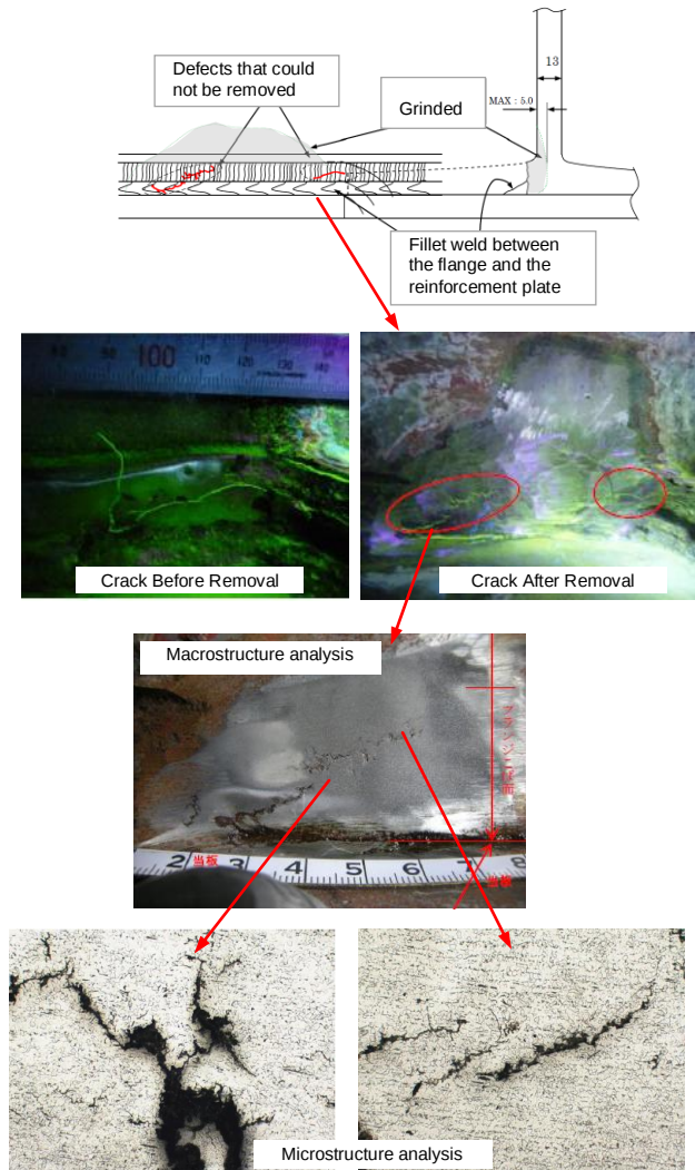
Figure 5: Conditions of the weld at the transverse beam after crack removal
