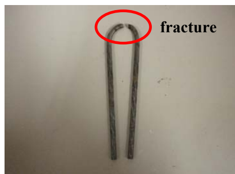
Photo 2: The fracture of PC rod
