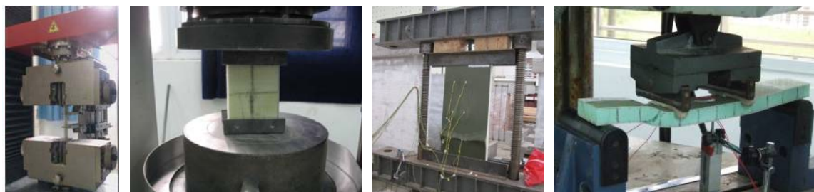
(a) Tensile test (b) Flatwise compression (c) Sidewal compression (d) there-point flexural test
