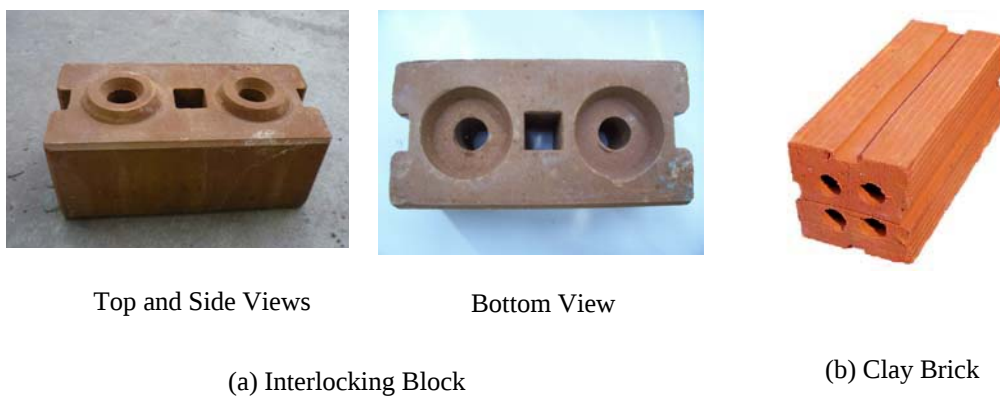
Figure 1: (a) The interlocking block and (b) the clay brick used in this study.
