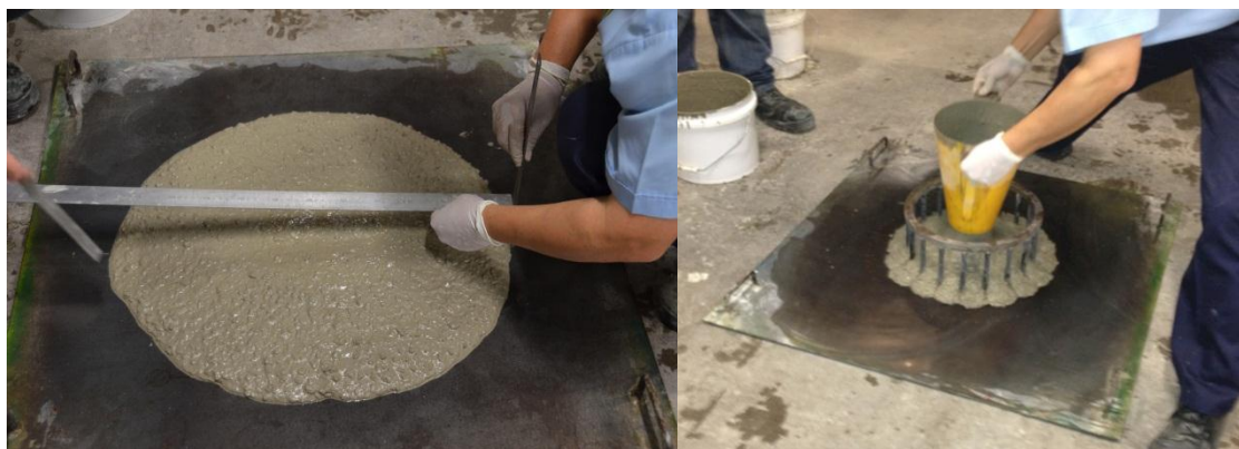
Figure 2: Slump-flow (on left) and J ring (on right) tests.
