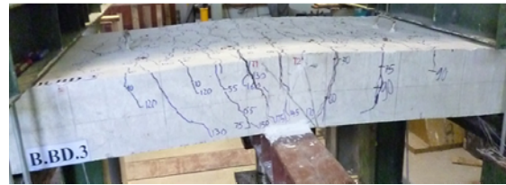
The bending failure of slab B.BD.3
