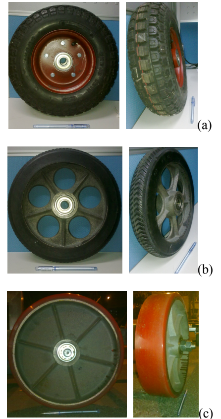
Fig. 2: Wheels: (a) inflatable, (b) rubber, (c) PU.
