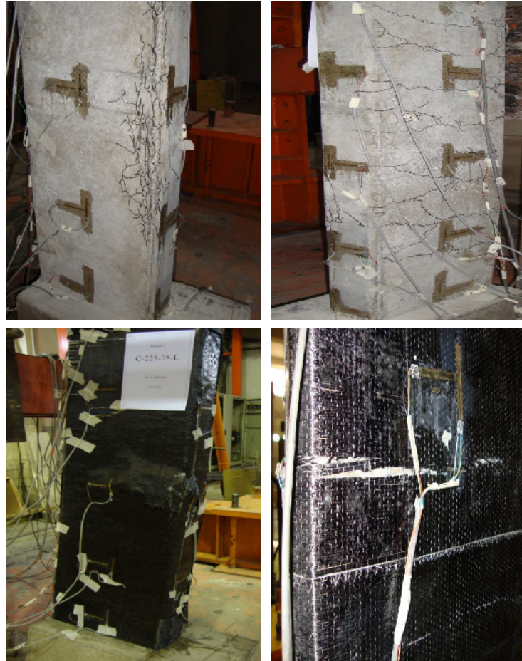
Figure 2: Failure and cracking pattern of unstrengthened and strengthened specimens
