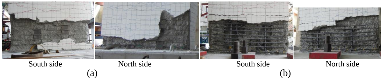
Figure 10: Comparison of failure mode (a) proposed pier (b) conventional pier
