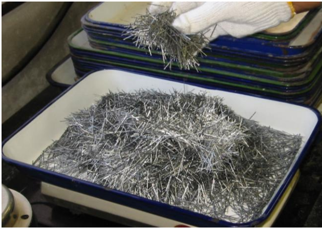
Figure 2 Sketch of the steel fibers
