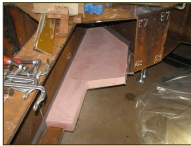
Photo 5: Plaster specimen at the inner surface of gusset plate
