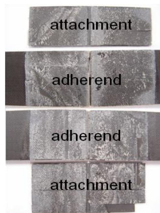
Fig. 4 Failure surfaces of SDLJ-2 sample
