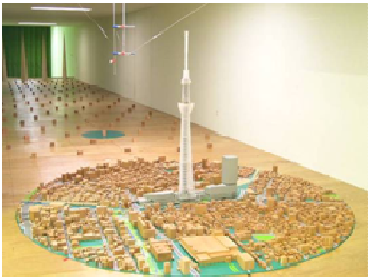
Figure 4: The entire wind tunnel test
