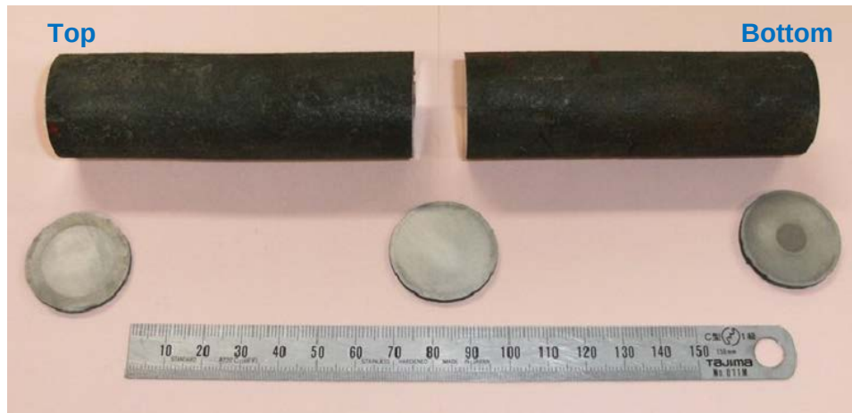
Fig. 6. An overview of extruded ODS316 bar.
