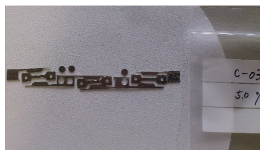
Fig. 4 Sub-sized sheet tensile specimens and TEM disks punched out from ribbon.
