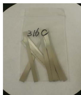
Fig. 2 Ribbons with 70-mm-length, 5-mm-width and 0.3-mm-thick.
