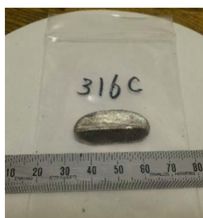
Fig. 1 Rod-shaped alloy button after forging at 1073K.
