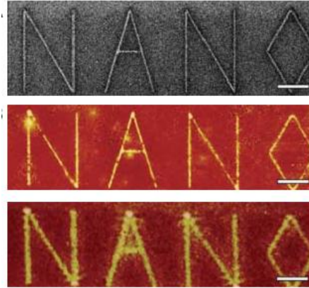
Figure 1.9 FIB and AFM image of object "NANO". 119
