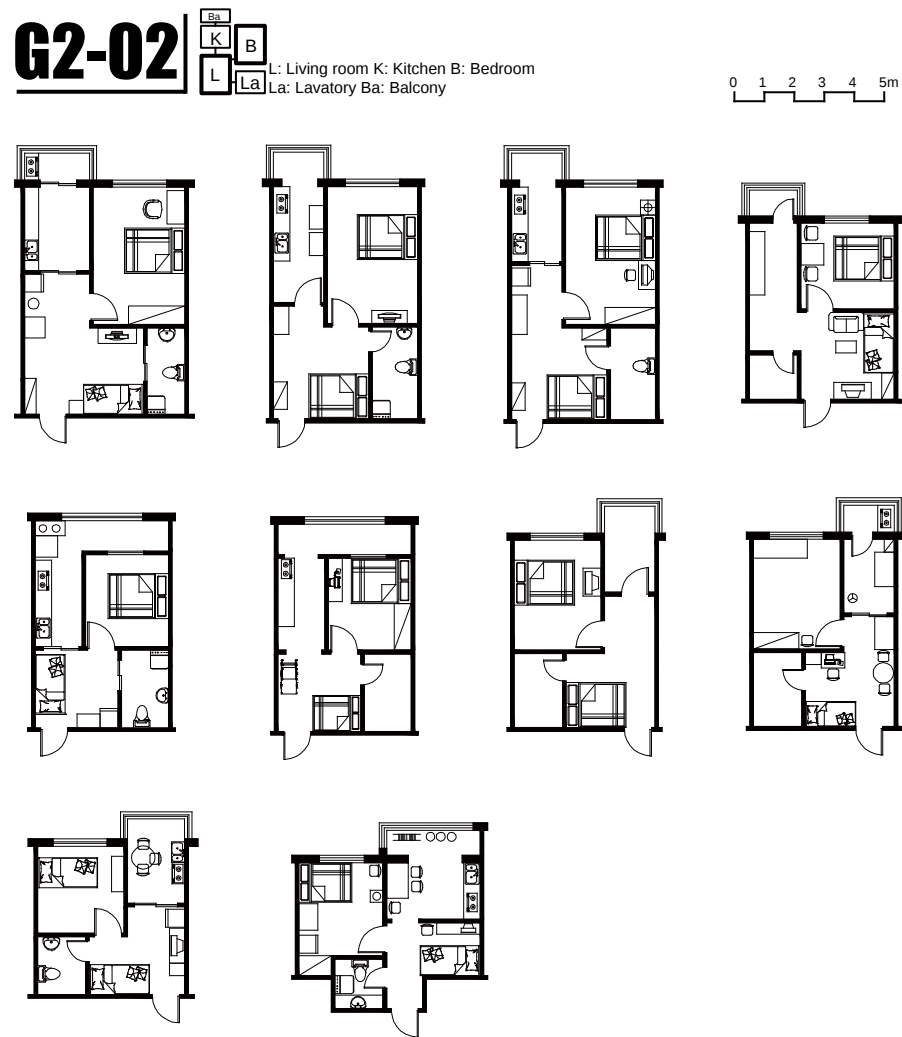
Figure 4-11 Room usage in G2-02
