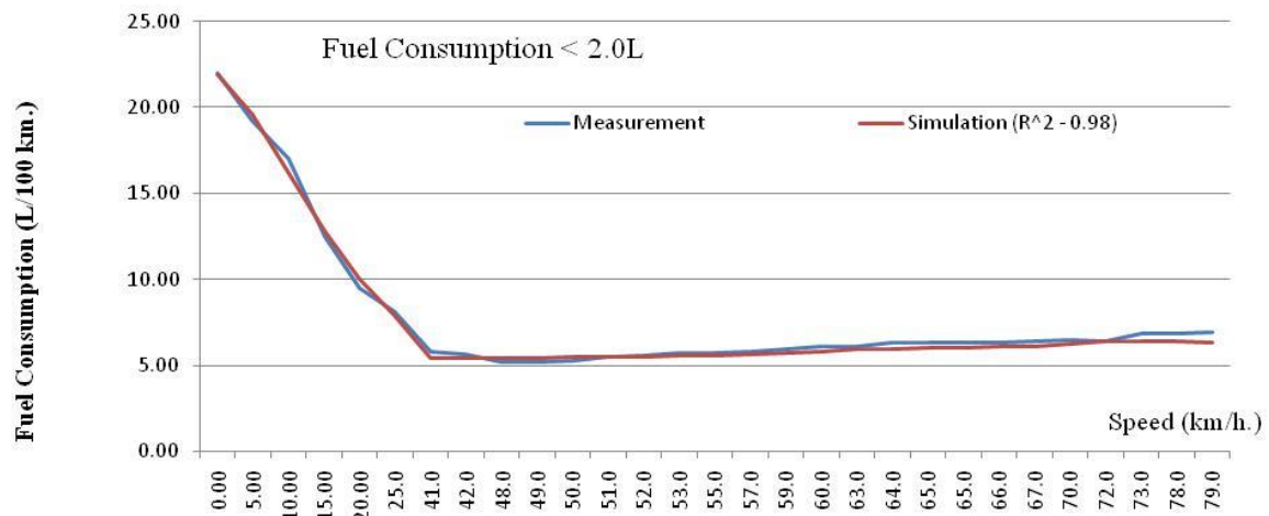
Figure 8.11 Fuel Consumption < 2.0L by Measurement compared with Simulated Model
