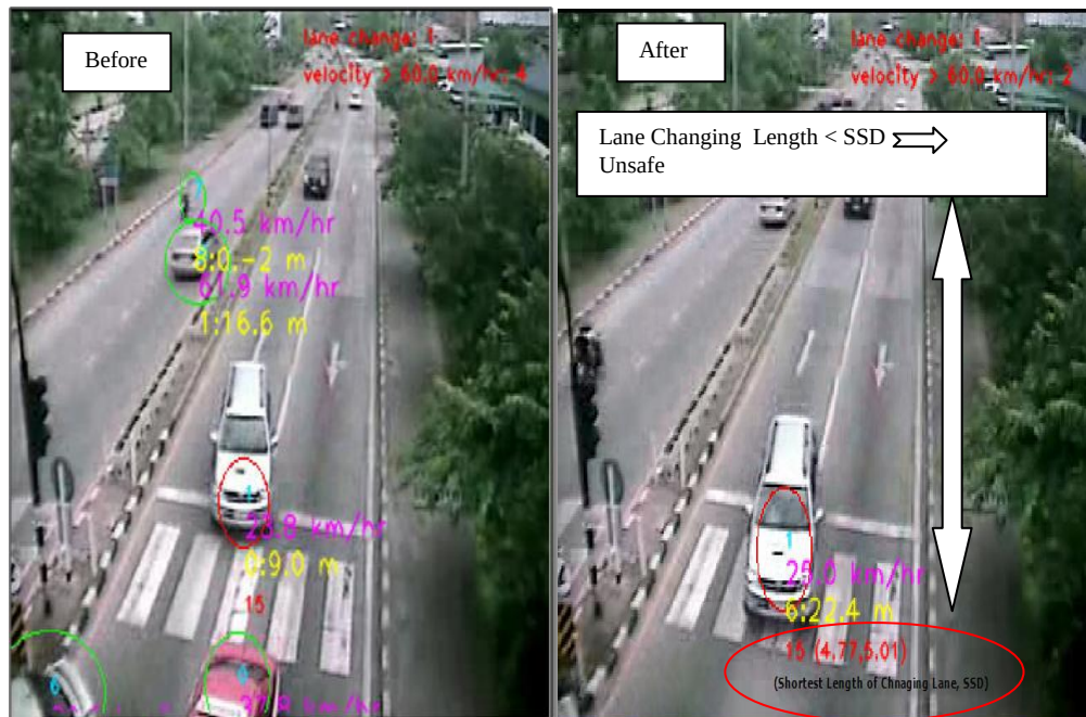
Figure 7.3 Degree of Lane Changing, Starting and Final Speed, Gap and SSD.
