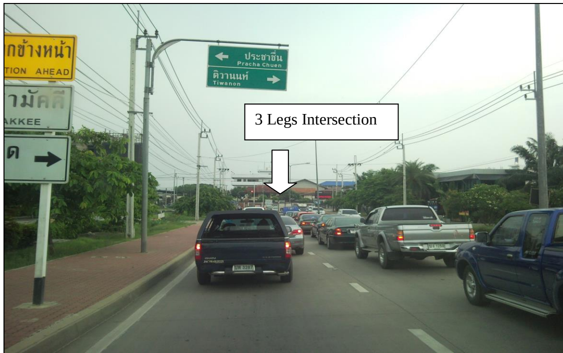
Picture 4.3 Queue Length at T Intersection is about 460 metres under the Fixed Times System.
