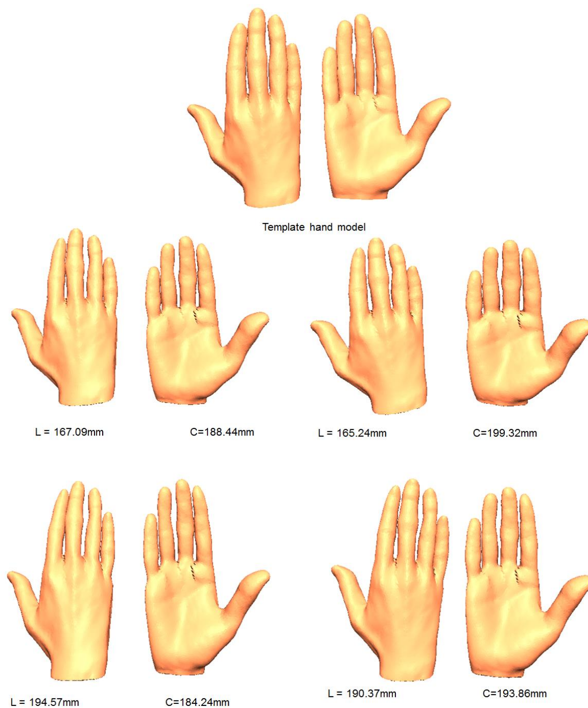
Fig. 5-8 Generated hand model instances with different major dimensions
