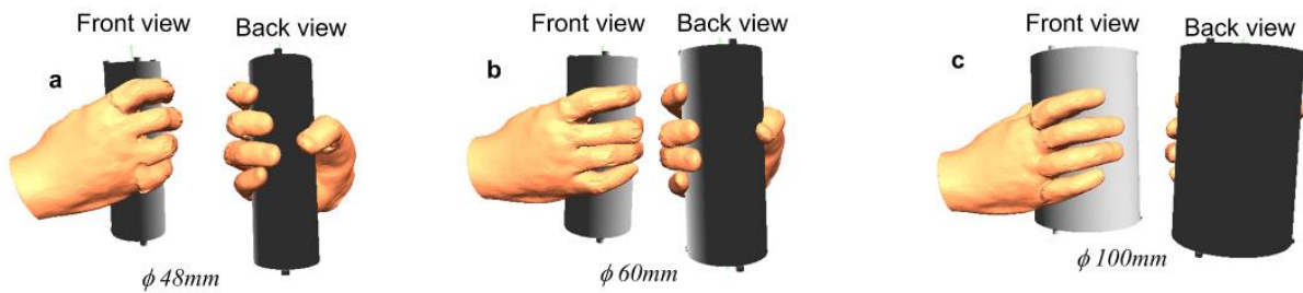
Fig. 3-19 Grasp posture generated by Digital Hand: (a) \phi 48\text{mm} cylinder, (b) \phi 60\text{mm} cylinder, and (c) \phi 100\text{mm} cylinder.
