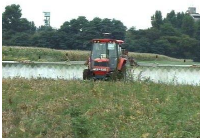
Figure 1-6 A robot tractor by using RTK-GPS and FOG (Kise et al. 2001)
