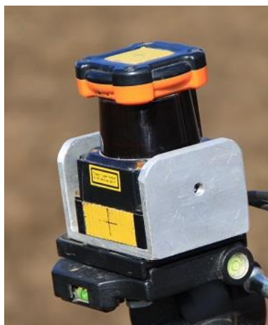
Figure 2-10 2D laser scanner (UTM-30LX)
