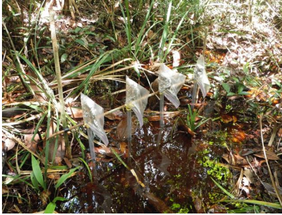
Fig. 6.2 View of field settings for dissolved CO 2 concentrations measurements at the study site.
