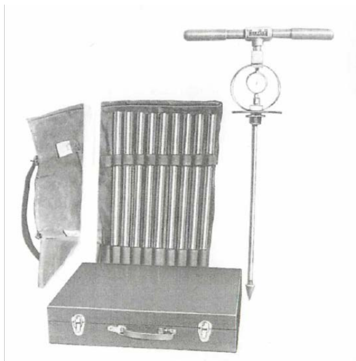
Figure 2-2 Cone penetrometer (MARUTO Testing Machine Company; Koga 2004).
