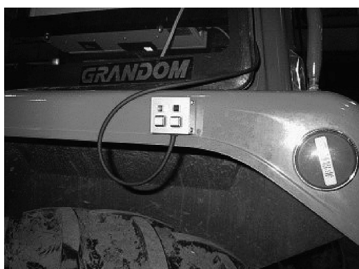
Fig. 7.2 The start and temporally stop switch (left) and emergency stop switch (right)
