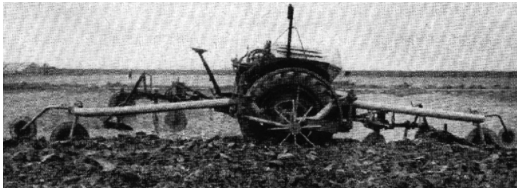
Fig. 1.2 “Agri-Robot”, unmanned plowing robot
