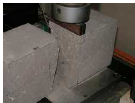
Fig. 5 Broken specimen by rectangular indenter.
