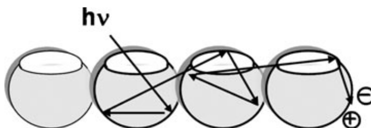
Figure 1.15 Application of the photonic crystal concept in an inverse opal configuration to increase the effective light path through the photocatalyst. Reproduced from Ref. 13.
