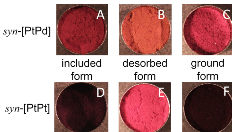
Figure 2-6. Photographs of powder samples: A and D) vapour-included forms; B and E) desorbed forms; and C and F) ground forms, for syn -[PtPd] and syn -[PtPt], respectively.
