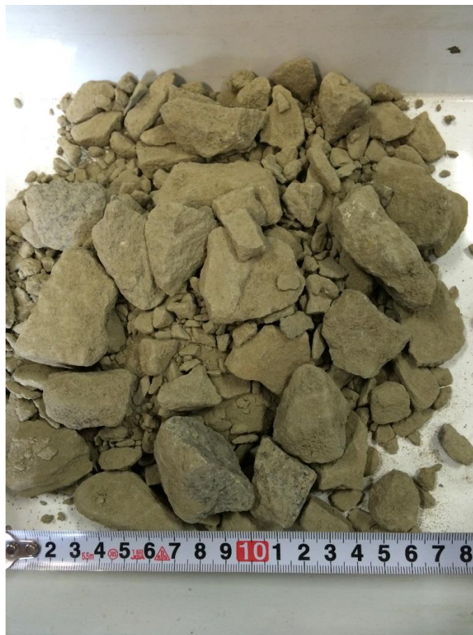
Figure 2-2 Photo of the granular subbase course material C-40.
