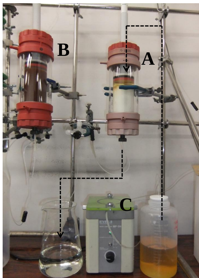
Fig. 2.2. Schematic diagram for the column system. A: DAX-8 resin column, B: Cation exchange column, C: Pump to draw solution into column. This picture shows the state of adsorbing DOM on DAX-8 resin. The DOM solution has yellow color (lower right), and the drain solution is clear (lower left).
