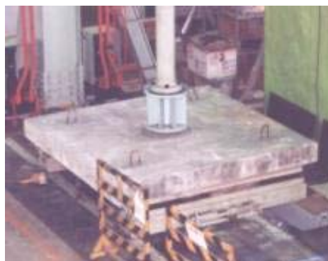
Figure 12 slab-type (two-directional sheet) dowel test [4]
