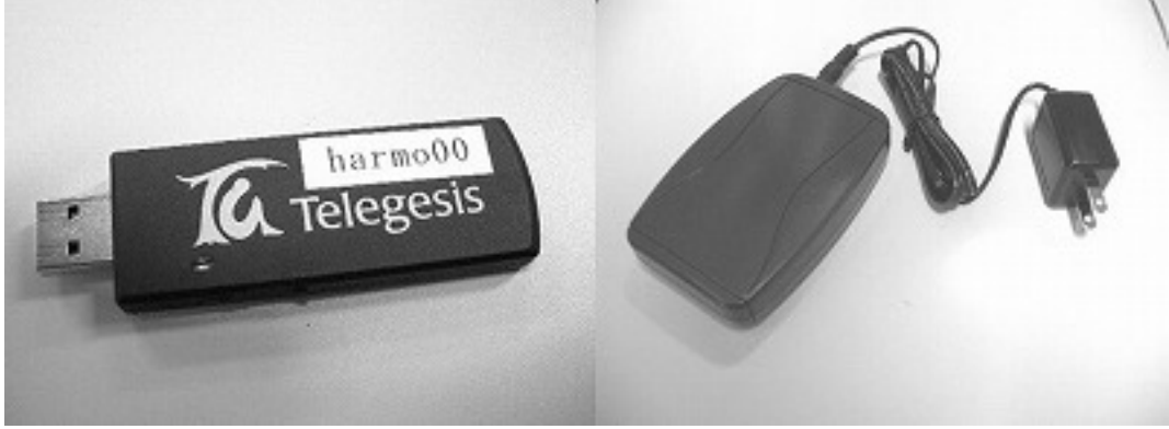
Figure 3.1: ZigBee modules: ETRX2USB (left), ETRX2 EAP-E (right).
