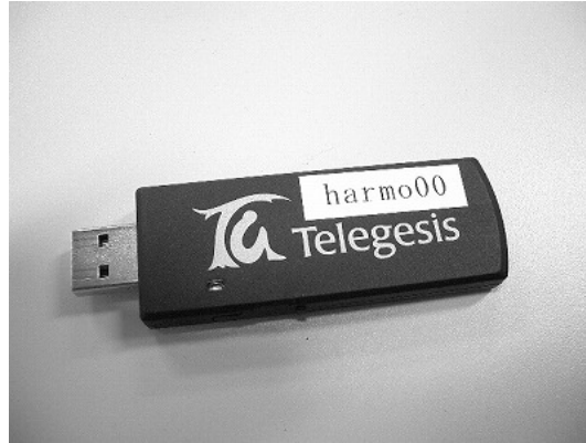
Figure 2.2: ZigBee node, ETRX2USB.
