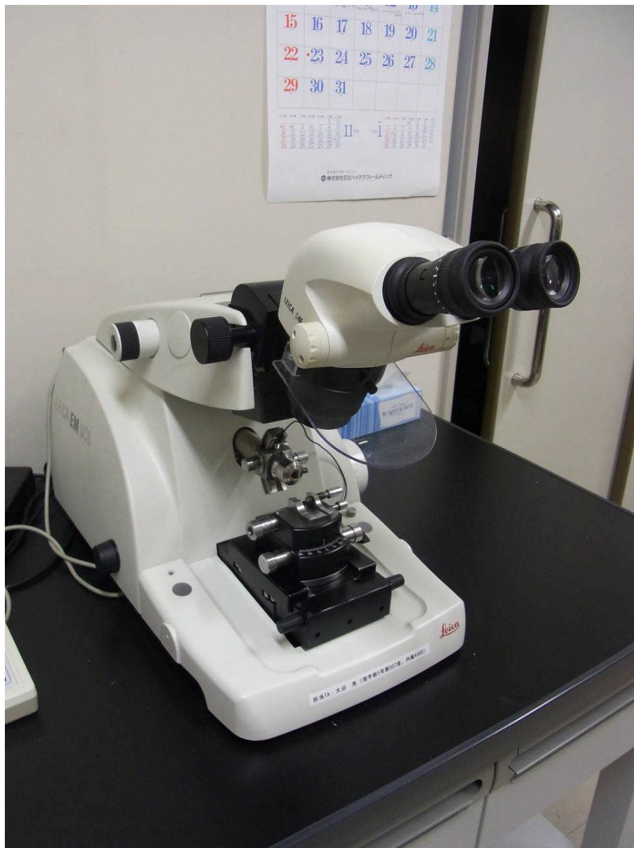
Figure 4-3. Photo of ultramicrotome EM-Supernova in division of biology, Department of Biological Science, in faculty of science in Hokkaido University.
