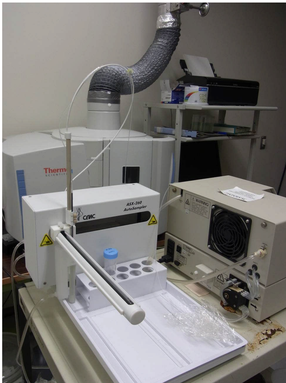
Figure 4-1. Photo of the inductively coupled plasma-atomic emission spectrometry (iCAP 6300 ICP Spectrometer) in Watanabe laboratory in faculty of science in Hokkaido University.
