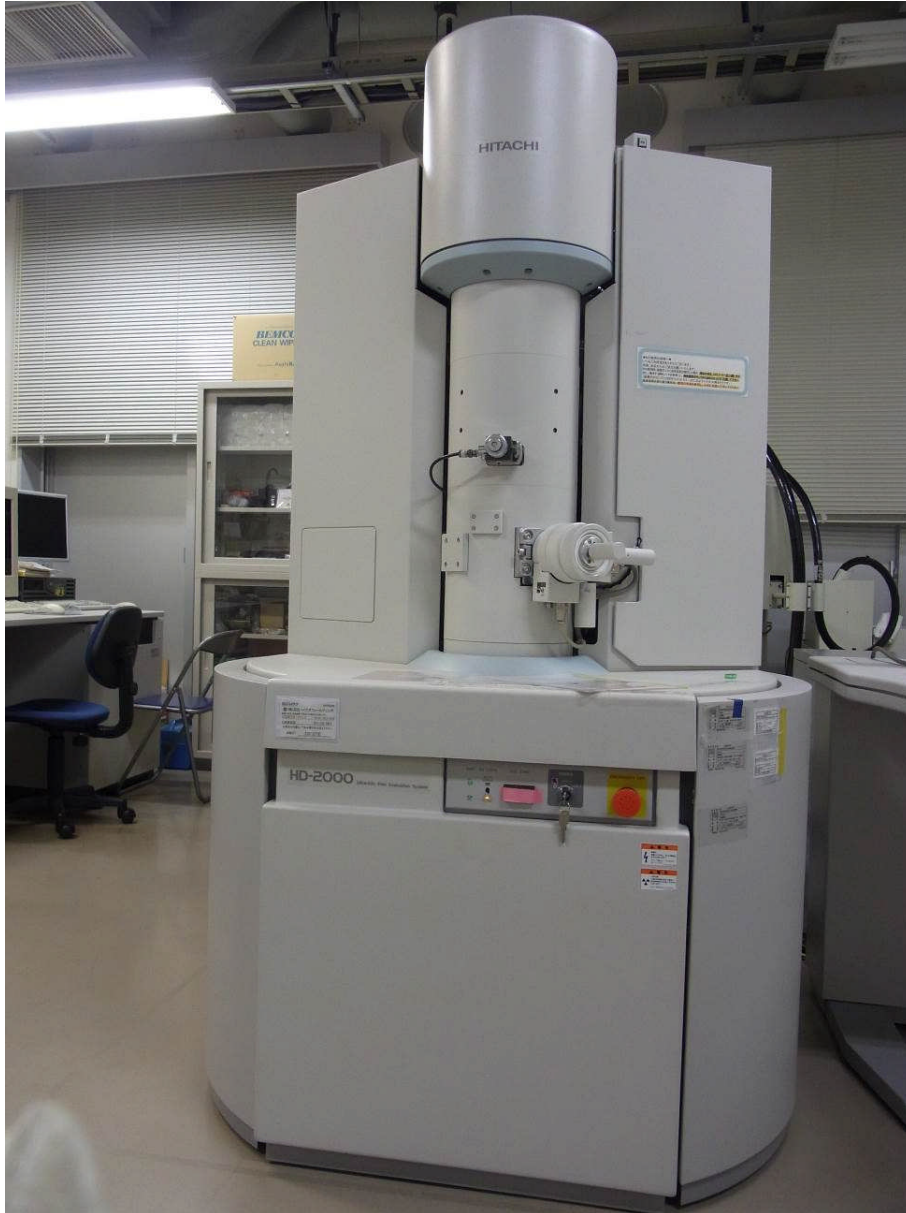
Figure 2-2. Photo of scanning transmission electron microscope STEM (HD-2000) with EDX (Genesis) in Creative Research Institution, Hokkaido University.
