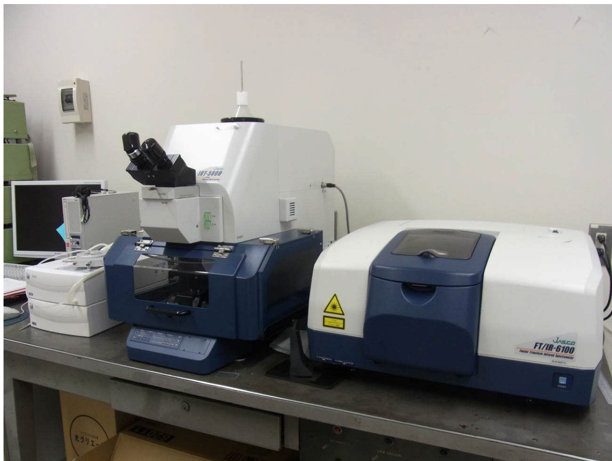
Figure 3-1. Photo of Fourier transform infrared spectrometer (FT-IR) installed in our laboratory.
