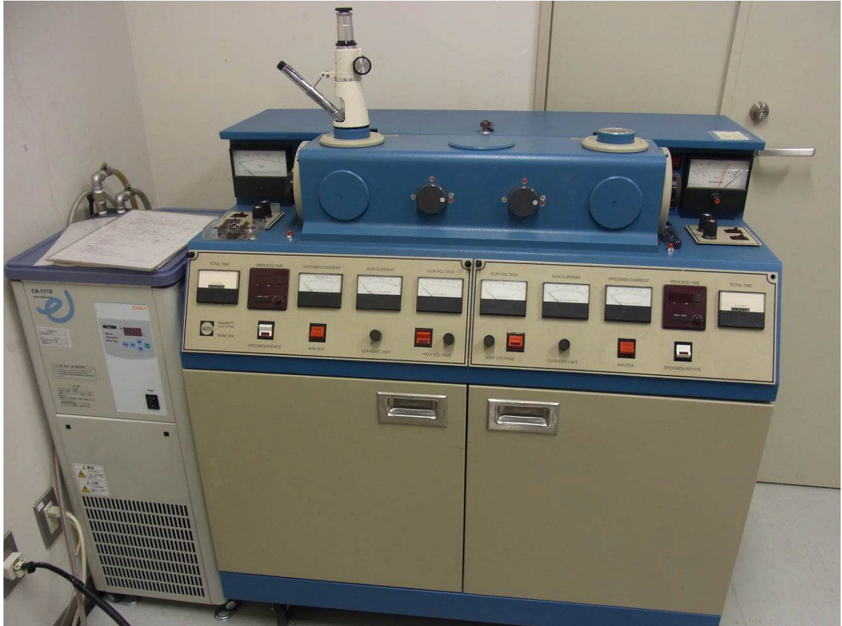
Figure 2-3. Photo of A Gatan Duomil 600 Ar ion milling apparatus in our laboratory.
