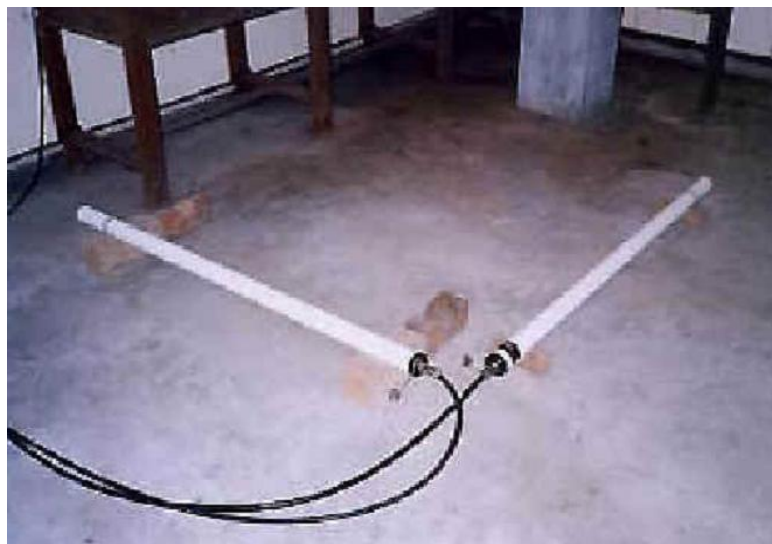
Figure 2.17. View of the magnetic search-coil antenna [Sato, 2004].
