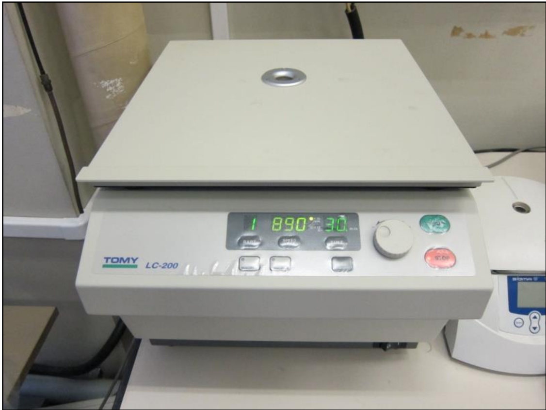
Figure 2-5 Tomy LC-200 centrifuge.
