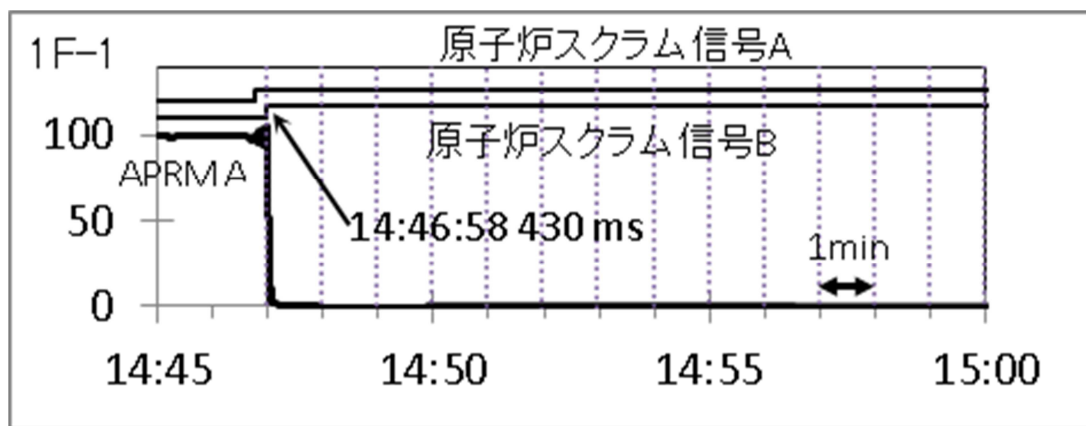
Fig. 2-3 Scram signal, APRM (Neutron Flux) (1F-1)
