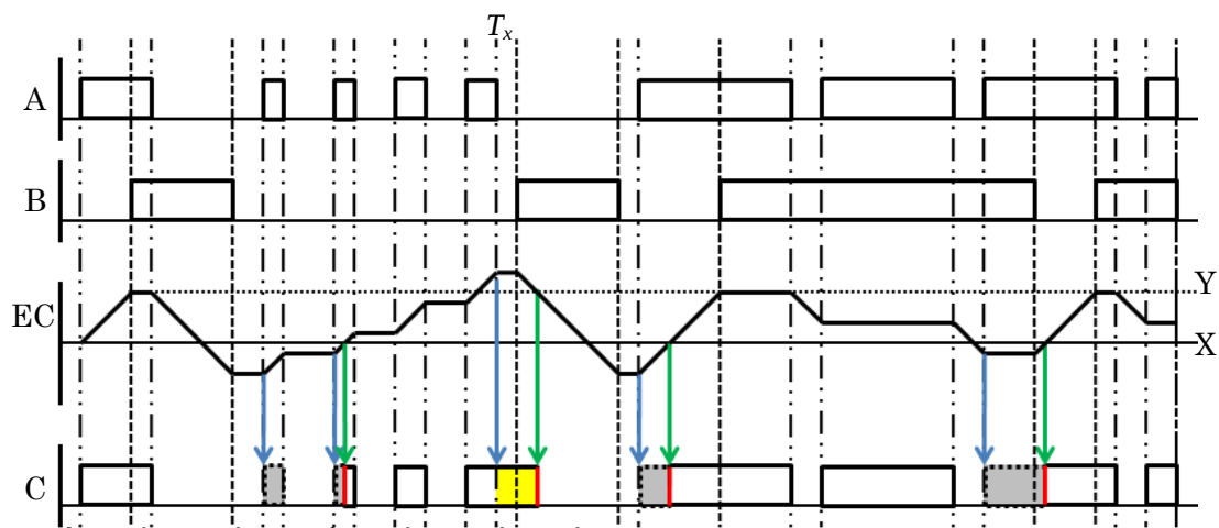
Fig. 3-18. Operation of proposed method(inputting short pulse)
