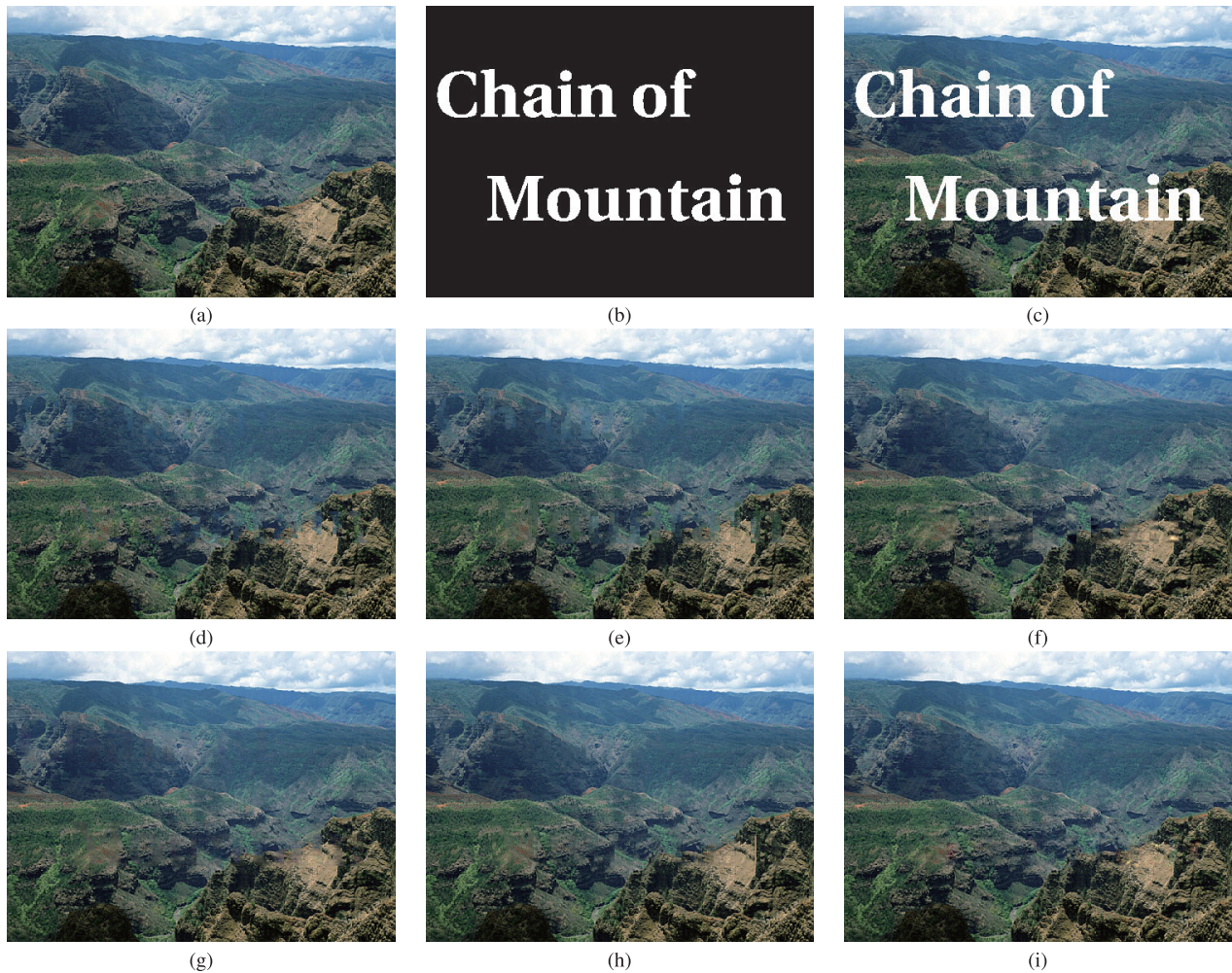
Fig. 2 Reconstruction results obtained from Image 1 by the previously reported methods and our method: (a) Original image ( 480 \times 360 pixels), (b) Flag image whose white regions correspond to missing areas, (c) Corrupted image including missing areas (8.9% loss), (d) Results by [9], (e) Results by [18], (f) Results by [12], (g) Results by [14], (h) Results by [21], (i) Results by the proposed method.
