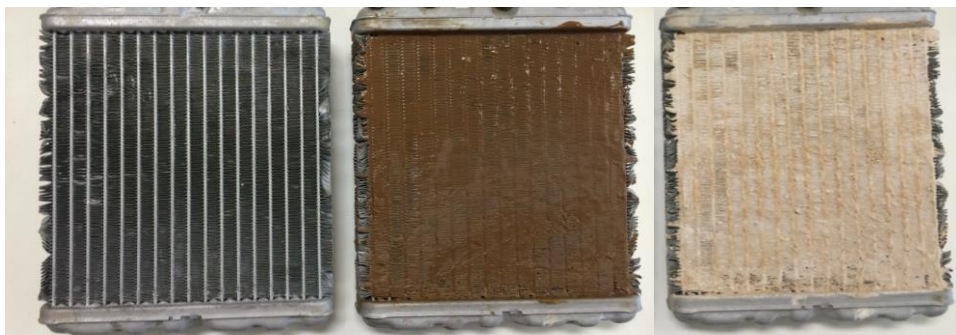
Fig. 6-1 Corrugated heat exchanger before being coated (left); being coated with slurry of WSS + 40 wt% LiCl (middle) and after coated (right)
