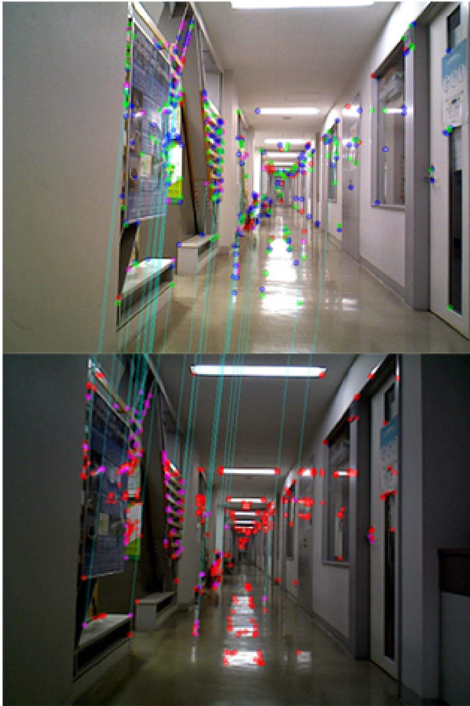
Fig. 6.7 Wrong feature matching: Wrong feature detected during the matching and are ignored.
