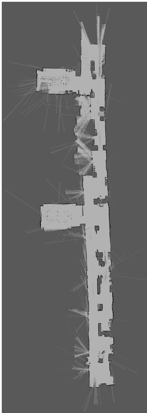
Fig. 5.20 The pose graph grid map is very accurate to the real environment
