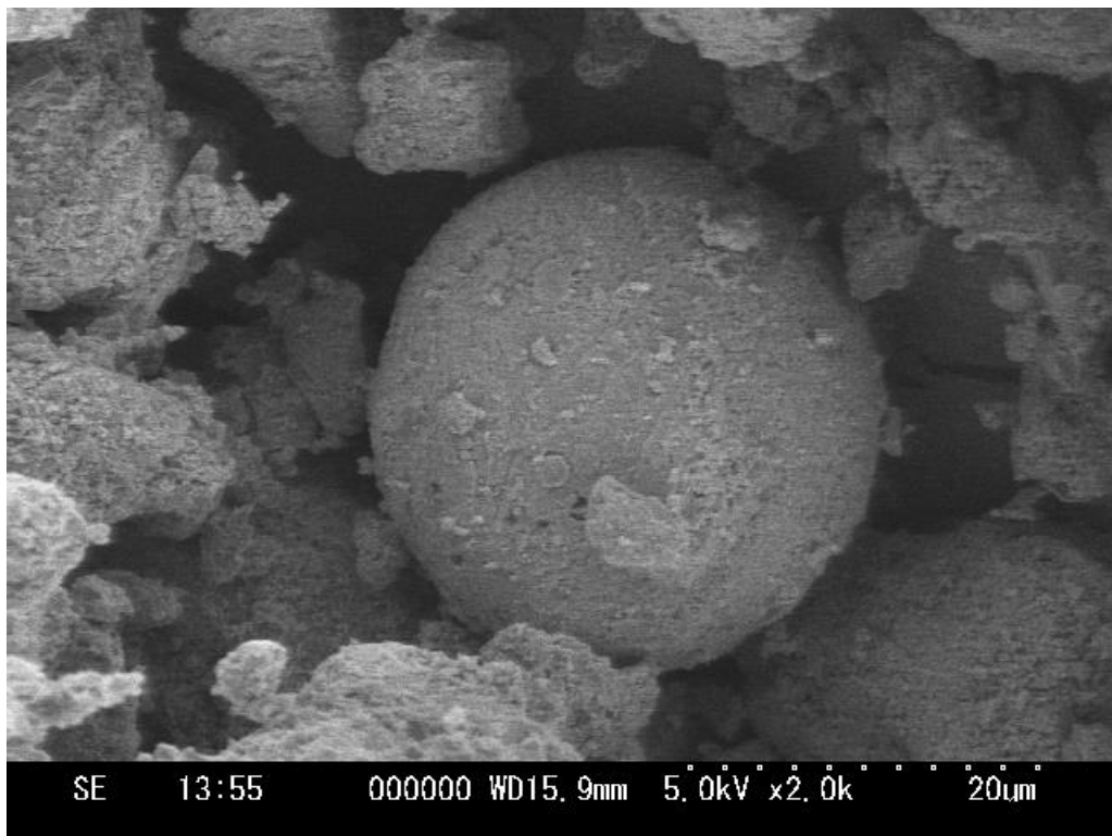
Figure 6.1: The presence of fly ash particle by Scanning Electron Microscope (Courtesy by Hokkaido Electric Power Co. Inc.)
