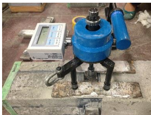
Figure 3-9 Direct pull-off test
