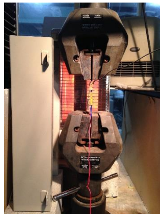
Figure A-1 Elevated temperature testing arrangement for the resin tensile test
