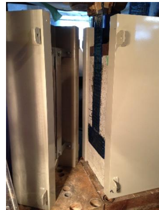
Figure A-2 Elevated temperature testing arrangements for the shear bond specimens
