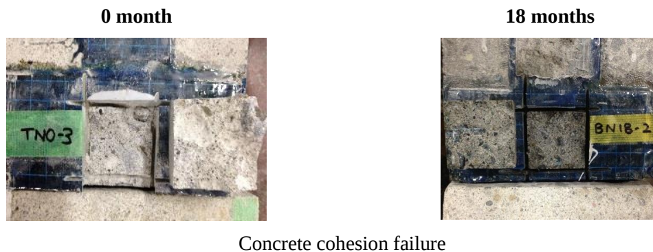
Figure 3-22 Comparison of typical failure mode before and after 18 months of exposure
