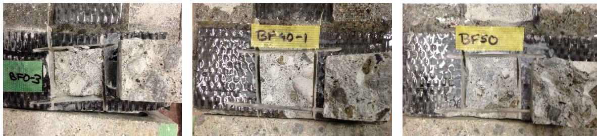
Figure A-13 Failure modes at 20 °C, 40 °C and 50 °C temperature respectively
