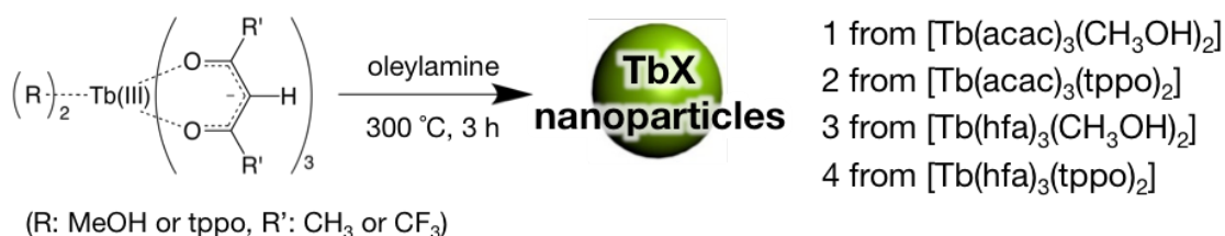
Scheme 5-5. Reaction scheme of TbX nanocrystals.
